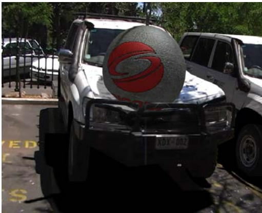
Figure 10: Inserting a synthetic object into video, using the known motion of the camera (see video attached to this paper). As the 3D shape of the car is known, it can interact convincingly with the object.
