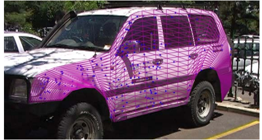
Figure 8: NURBS surface fitted to reconstructed object points.
